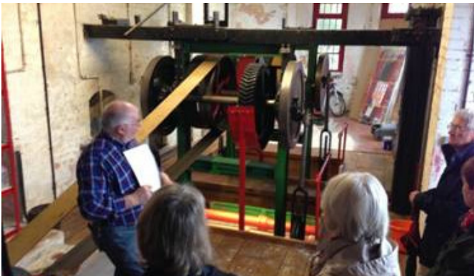
The pump room October 2013. Note the chevron cog wheels, the construction of which was patented by Andre-Gustave Citroen and the chevrons used as the company logo.
